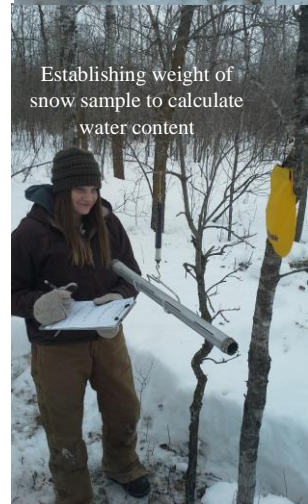
Obtaining snow depth and core sample
